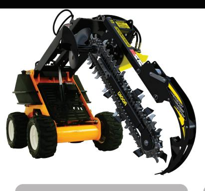
Designed specifically for mini loaders and walk behind machines, the Digga Mini Bigfoot Trencher is the lightest, most compact, powerful mini trencher on the market today. Unique design gives the operator consistent digging depth, efficient spoil to one side of the trench and finely crumbed spoil for effective compaction back into the trench. Provides minimal ground disturbance to surrounding conditions and a cleaner job finish.
